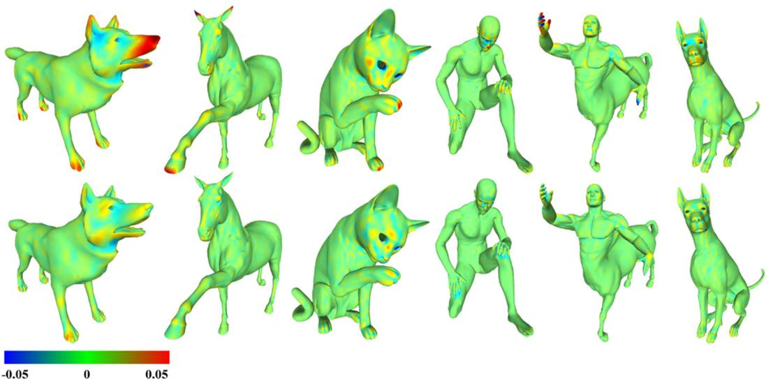
**Fig. 4.** Visualization of signed distance between each result ( $N_{res}/N_{org} = 0.05$ ) and original mesh. Upper row is the QEM result, Lower is the result of the proposed method. Red and blue areas denote regions far from the original mesh, signifying damaged shape. Green areas indicate close proximity to the original shape, showing minimal deviation
